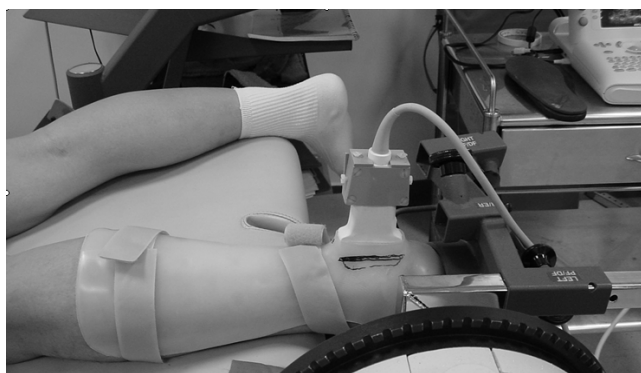
Figure 1: Experimental setup for the dynamic ultrasonic measurement of the Achilles tendon.
