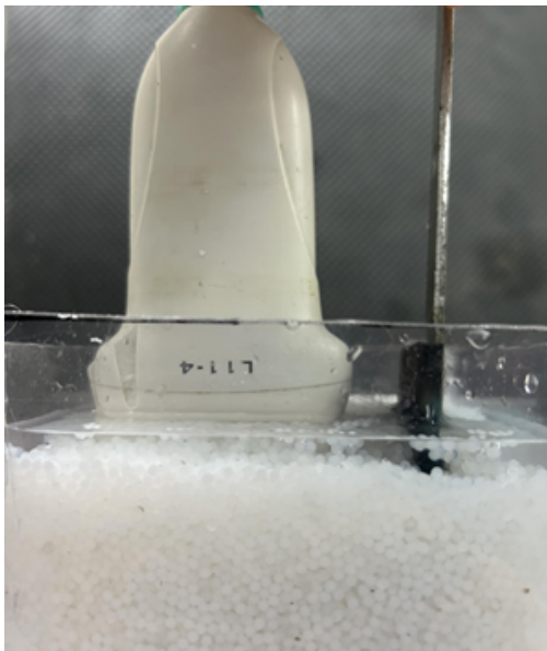
Figure 1: A 128-element ultrasound probe controlled by a Verasonics scanner allows measuring the response of the granular medium. The 1 mm diameter spherical silicon beads are saturated with water. Plane waves are generated with a corrugated plate attached to a vibrating exciter. Frequency ranges from 50Hz to 700 Hz
