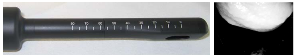
Figure 1: (a) Aspiration probe: Modular tip with the aspiration cavity. (b) Camera view of the aspirated tissue.
