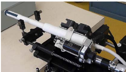
Figure 1: Modified stepper with shaker and probe.
